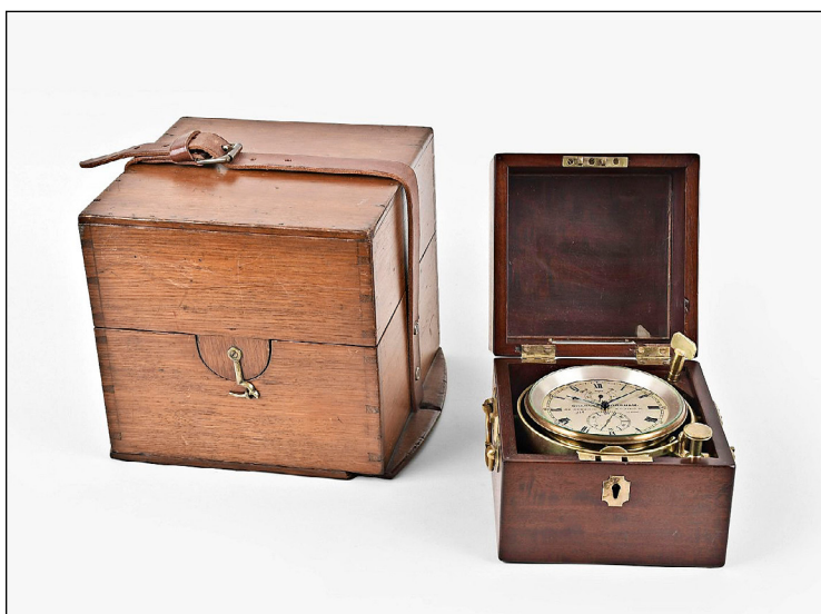
Charles Frodsham, London, produced this mid-Nineteenth Century two-day marine chronometer. It was one of several navigating instruments in the sale. It had a fusee movement and a silvered dial with wind indicator. It earned $3,120.
